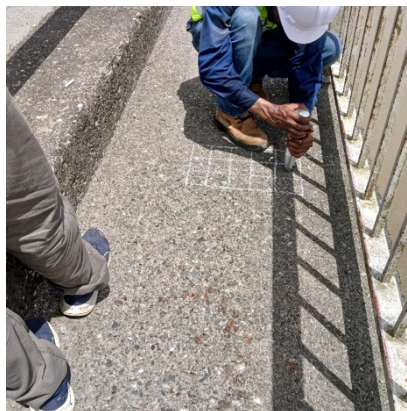
Fig. 2 Vertical position of the plunger during hitting the concrete surface.
