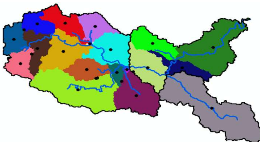
Fig. 2. Subcatchments in Wadi Dayqah Watershed developed using HEC-HMS
