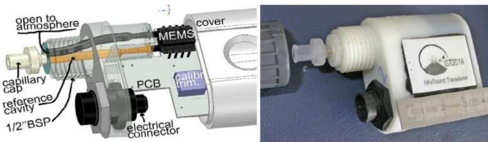
Fig. 3. Left: Schematic block diagram of the infrasound sensor, illustrating the key components including the MEMS microphone, capillary tube, reference cavity, electronic board, and connector. These elements are assembled within the protective housing shown in the right panel [Grangeon et. al.].
